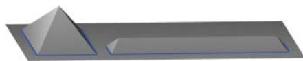
Fig. 1. RV is calculated by substituting DTR for elevation and then calculating the volume beneath the pseudotopographic surface. Two examples are shown, with perimeter roads in blue (there is a hidden road along the back of each volume). (Left) For a 1-km-square road pattern, the pyramid has a height of 0.5 km and a volume of 0.167 km 3 . (Right) The elongated pyramid measures 0.333 by 3 km and therefore has the same footprint area as the square pyramid, but its volume is 47% of the square pyramid volume. RV simultaneously accounts for area and shape.
